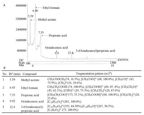
Figure 2: GC-MS spectrum of CA (A) and fragmentation pattern (B), aRetention time (min), mass/charge relation (m/z).
