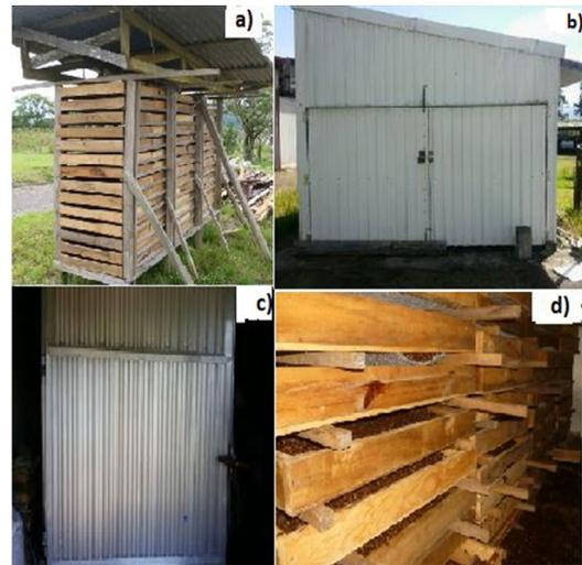
Figure 1 – Devices designed for samples drying: air drying (a); a 6 m<sup>3</sup> capacity solar dryer (b); experimental (conventional) NARDI dryer (c) and stacked trays with gaps to allow air circulation (d).
