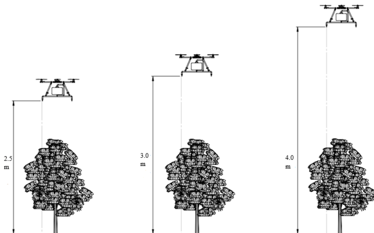
Figure 2. Schematic of pesticide application in the coffee plantation at a flight height of 2.5 m (A), 3.0 m (B), and 4.0 m (C)
